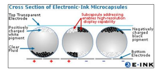
Figure 3. Principle of electronic paper, courtesy of E-ink Technology.
